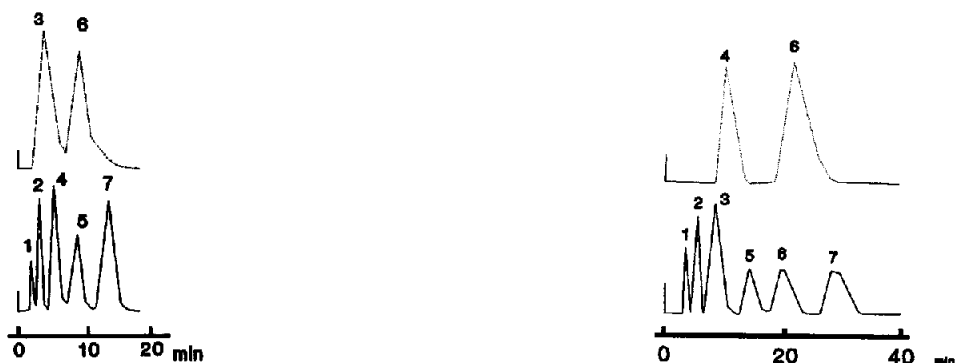
Fig. 2. Chromatogram of a solution of 2 ppm F^- (1), 5 ppm Cl^- (2), 3 ppm S^{2-} (3), 25 ppm NO_3^- (4), 50 ppm HPO_4^{2-} (5), 6 ppm SO_3^{2-} (6) and 50 ppm SO_4^{2-} (7). Column, 100 \times 3 mm (Oka-1). Eluent, 0.0025 M sodium carbonate (1 ml/min). Solid line = conductimetric detector output; dotted line = spectrophotometric detector output.
